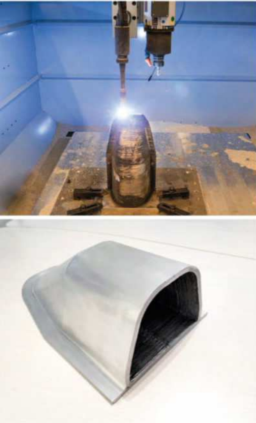
▲ A combination of 'metal additive' 3D printing with CNC 'subtractive' routing can result in cost-effective products, such as this vent cowling created by a Diversified Machine System (DMS) hybrid
