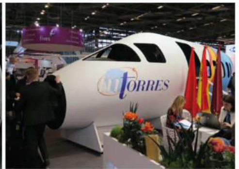
▲ Composites are replacing traditional metal constructions where lightweight, high tolerance and anti-corrosion properties are paramount, such as with this monocoque aircraft fuselage from M.Torres Disenos Industriales SAU. A tooling reduction of up to 70% is claimed
