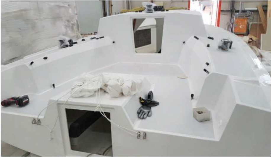
▲ The Loop 650 from GS4C SRL is a 'cradle-to-cradle' composite sailing vessel designed to be fully recyclable, hence avoiding the 'cradle-to-grave' element
