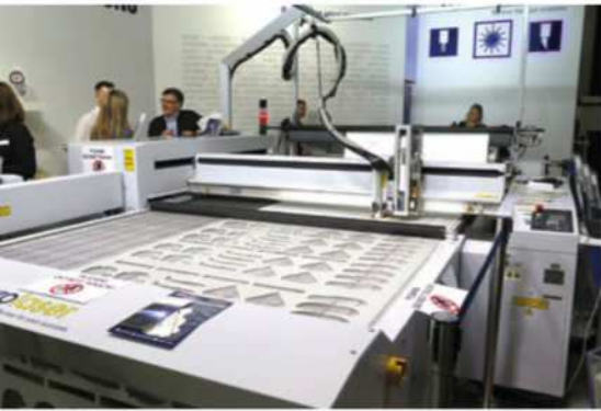
▲ Precision cutting of reinforcement cloth, especially carbonfibre, minimises waste and helps pay back the investment in the machine
