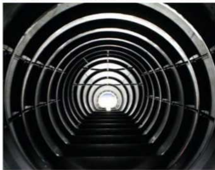
▲ Composites are replacing traditional metal constructions where lightweight, high tolerance and anti-corrosion properties are paramount, such as with this monocoque aircraft fuselage from M.Torres Disenos Industriales SAU. A tooling reduction of up to 70% is claimed
